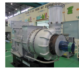
Mixed hydrogen combustion turbine
