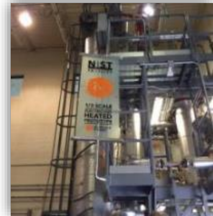
One-third scale NIST-1 Test Facility
