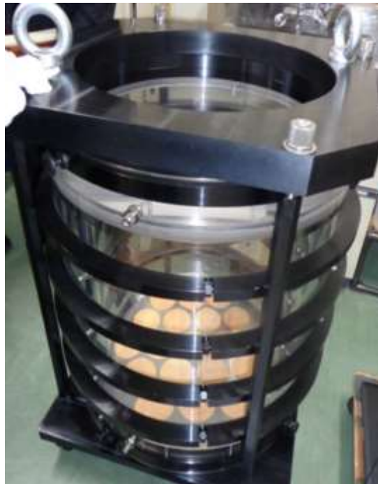
Figure 1-11. Design of the apparatus (from presentation by Kajima 15th meeting on re-saturation of bentonite).
