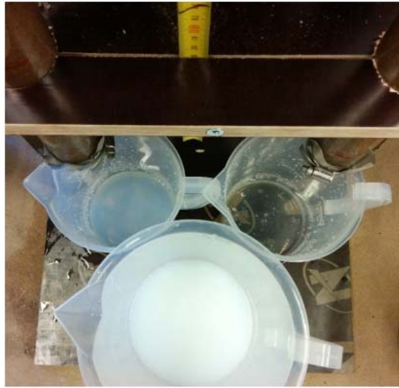
Fig.-10 In a can in the forefront of the picture is colloidal silica that was used during the tests. A can on the right side of the picture is placed under the pipe filled with artificial groundwater and based on the colour of the liquid in the can it can be assumed that silica did not penetrate through the sand layers. In the can on the left side of the picture, there is also some silica that penetrated through the sand layers among the fresh tap water.
