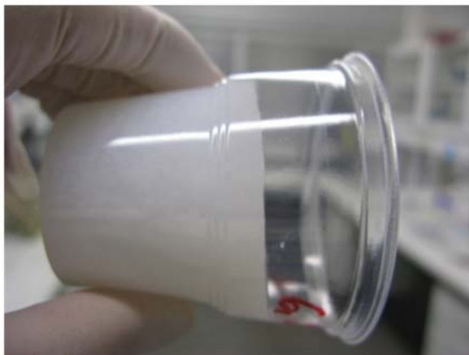
Fig.-2 Fulfilment of gelling criterion during cup test.
