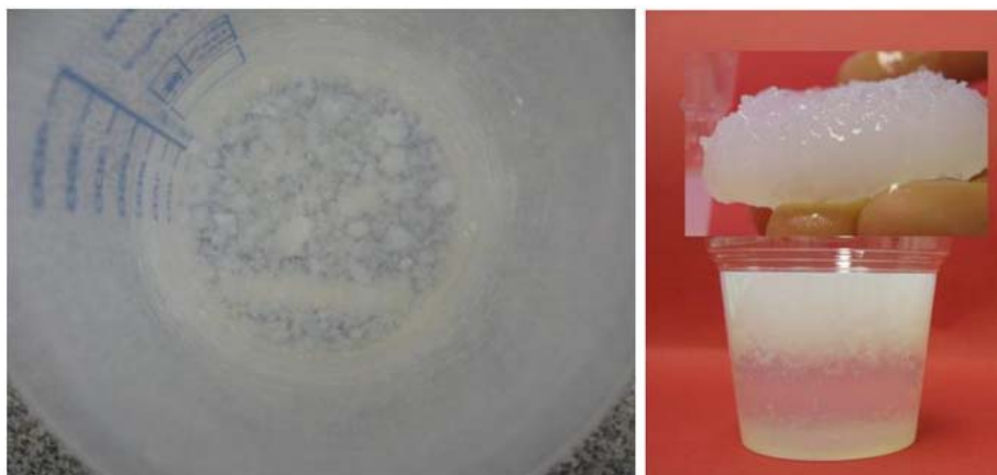
Fig.-3 On the left, flocculation during mixing caused by calcium. On the right, two different phases of gel prepared from calcium chloride with ionic strength 0.45 M immediately after mixing. Also, a solid phase that appeared on the surface of the mixture can be seen on the picture.
