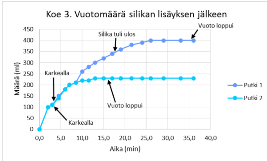
Fig.-12 Leakage volume after adding silica in test 3. In pipe 2 that was saturated with an artificial groundwater, penetration was clearly weaker than in pipe 1 as 170 ml less of colloidal silica flowed through the pipe 2. 2
