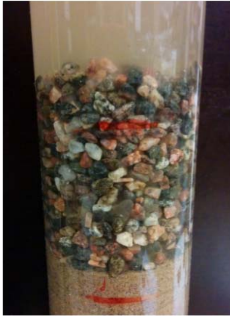
Fig.-9 Pipes were completely saturated with water. Water poured on the layer of sand with grain size equal to 2,0...4,0 mm was muddy after mixing with sand dust.
