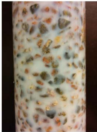
Fig.-16 Flocculation of silica particles in pipe 2 due to the salinity of artificial groundwater. Picture from test 5.
