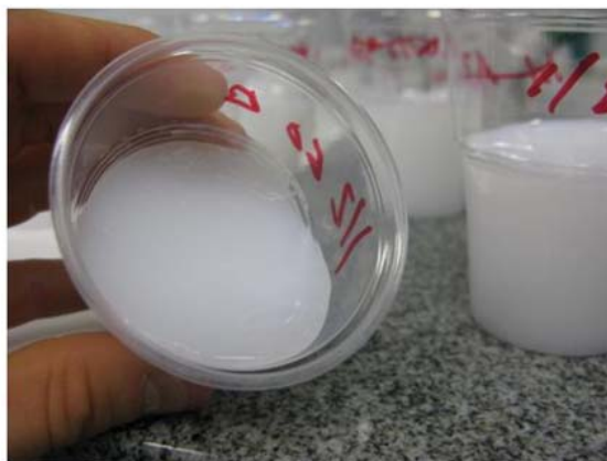
Fig.-4 Gel from diluted silica sol one day later after mixing. Reference mixture, its silica content was reduced by a half and was exposed to 60 ml of groundwater.
