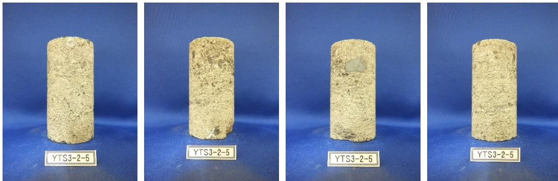
熱伝導率測定供試体⑤ (110°C 炉乾燥状態)
