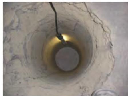
d) Filter frit at top of seal
